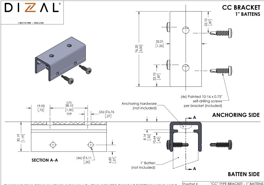
Recommended Span distance mounting for anchor screws (by others) and/or DIZAL Brackets is 8'-0" [2438mm] center to center\*. \*Calculated for 1" [25mm], 1.5" [38mm] and 2" [50mm] battens thickness from 2" [50mm] to 8" [203mm] width. For other dimensions, please contact us at info@dizal.com. NOTE: The first screw/bracket must be installed a maximum of 12" [305mm] from the batten end. IMPORTANT: Always check local building regulations before installing DIZAL battens.
