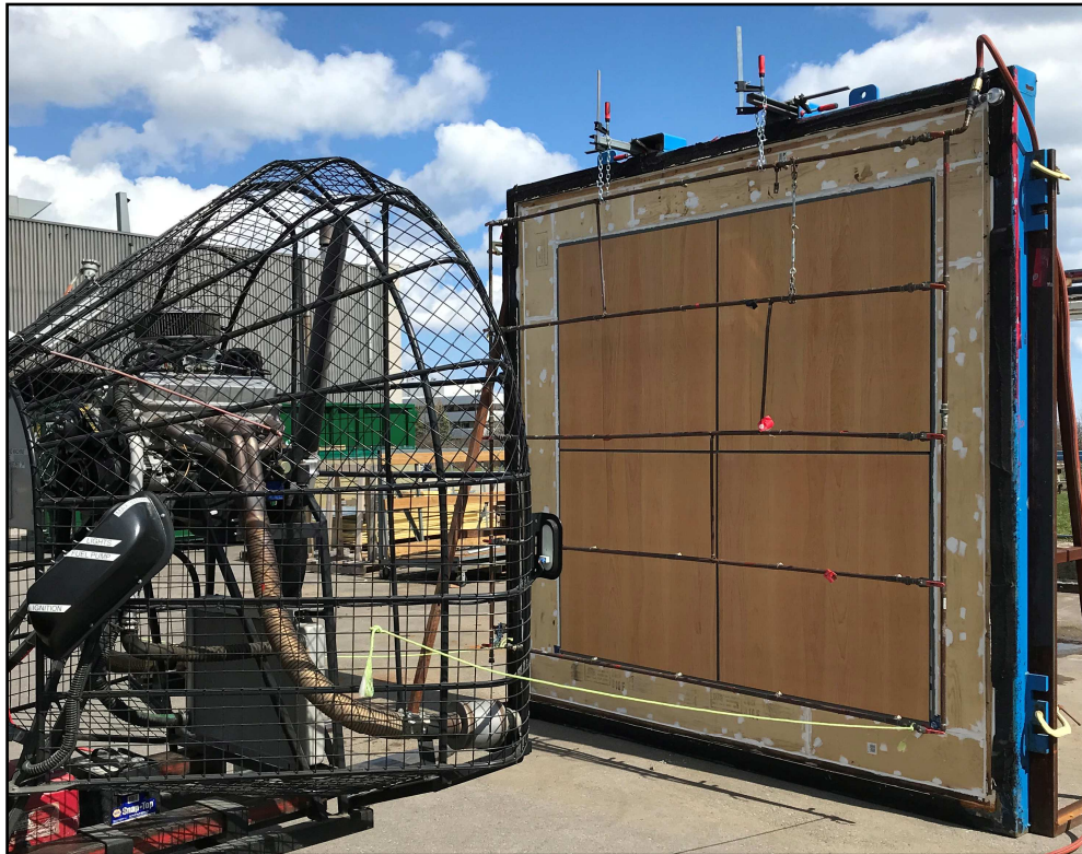
Figure 5 – AAMA 501.1, Dynamic Water Penetration Test
