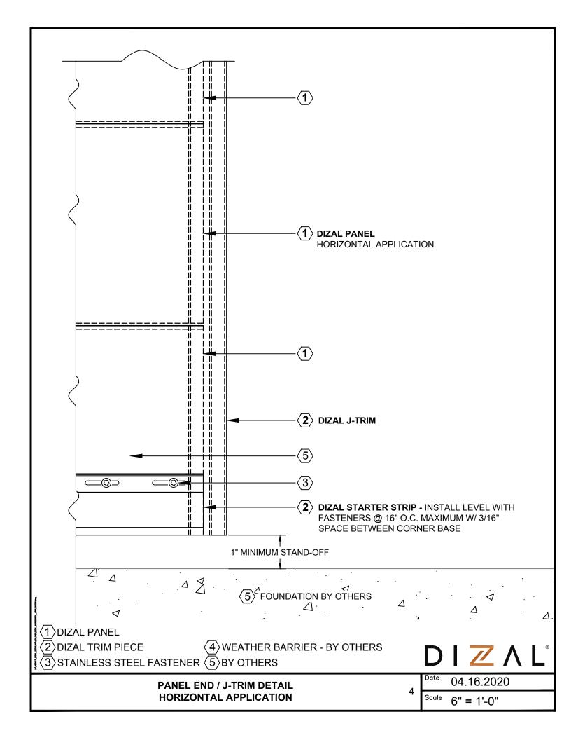
KEEP 3/16" BETWEEN THE TRIM AND THE PLANK TO ALLOW FOR EXPANSION AND CONTRACTION.
