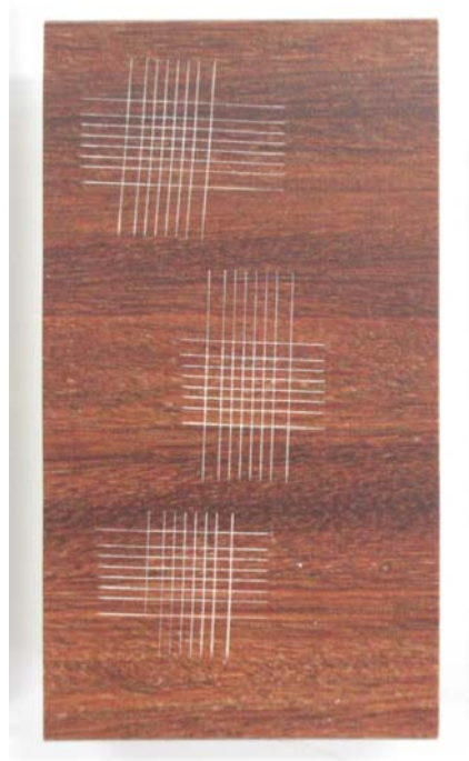
Sample after adhesion test
