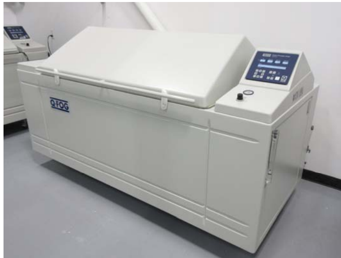
Salt Fog/Spray machine used
